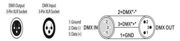
For installations where the DMX cable must be operated over long distances or electrically operated in a noisy environment, such as in a disco, DMX termination is recommended. This helps prevent electrical damage to the digital control signal noise. The DMX terminator is only connected between the XLR plug pins 2 and 3 of the  $120\Omega$  resistor and then inserted into the output of the last fixture. The XLR socket is in the chain. Please see the illustration below.
