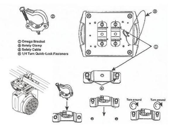
Regardless of the rigging option you choose for HAWKEYE II, always be sure to secure your fixture with a safety cable. The fixture provides a built-in rigging point for a safety cable on the hanging bracket as illustrated above. Be sure to only use the designated rigging point for the safety cable and never secure a safety cable to a carrying handle.
