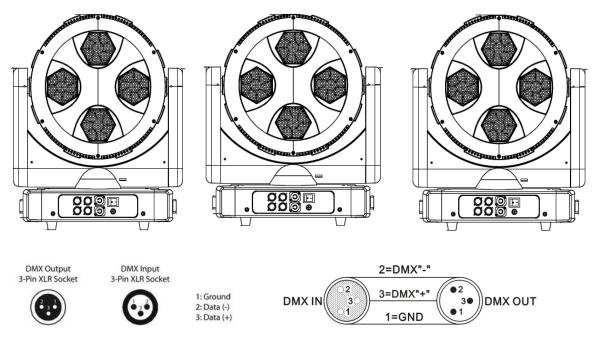
For installations where the DMX cable has to run a long distance or is in an electrically noisy environment, such as in a discotheque, it is recommended to use a DMX terminator. This helps in preventing corruption of the digital control signal by electrical noise. The DMX terminator is simply an XLR plug with a 120  $\Omega$  resistor connected between pins 2 and 3,which is then plugged into the output XLR socket of the last fixture in the chain. Please see illustrations below.
