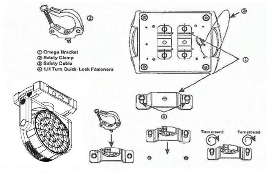
Regardless of the rigging option you choose for our fixture, always be sure to secure your fixture with a safety cable. The fixture provides a built-in rigging point for a safety cable on the hanging bracket as illustrated above. Be sure to only use the designated rigging point for the safety cable and never secure a safety cable to a carrying handle.
